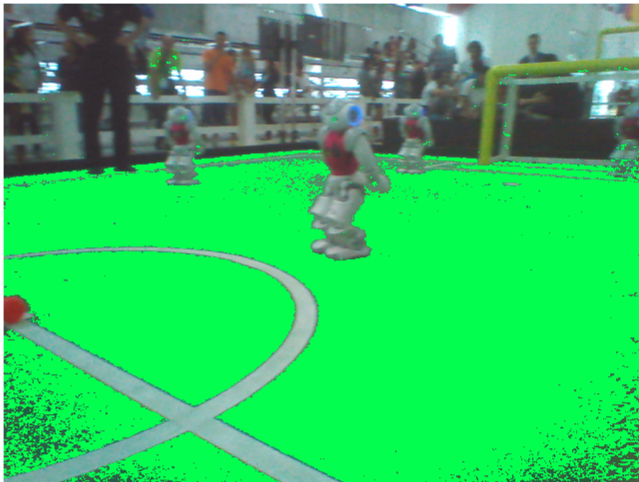
Figure 3: Automatically detected field color
