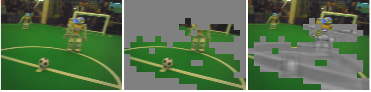
Figure 10: Hypotheses Generation, original image (left), low contrast / above field border regions (center, grey), CB-channel difference within high contrast regions (right, grey)
